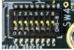
Figure 4. ILC150E Configuration Switch SW4
