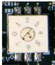
Figure 6. ILC150E Configuration Rotary Switch SW3
