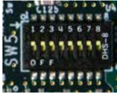
Figure 5. ILC150E Configuration Switch SW5
