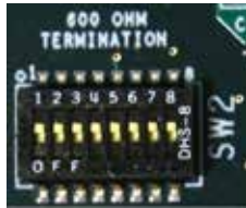
Figure 3. ILC150E Configuration Switch SW2
